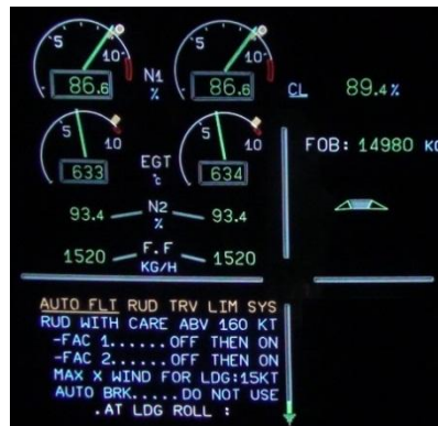
Figure 34: The ECAM messages after RTLU 1 and 2 fault
