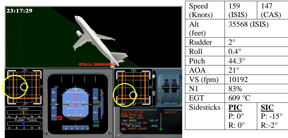
Figure 27: The aircraft attitude at the highest pitch angle
