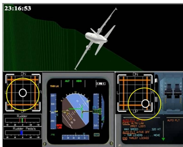
Figure 25: Aircraft rolled 54° to the left
